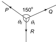
2. A body is in equilibrium under the action of three coplanar forces  $P$ ,  $Q$  and  $R$  as shown in the figure. Select the correct statement
